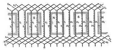
F1G. 80. Diagram of wave winding for d. c. armature as used in railway and other motors and some generators.
